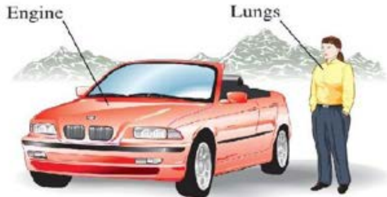
FIGURE At high altitudes, a car engine generates less power and a person gets less oxygen because of the lower density of air.
