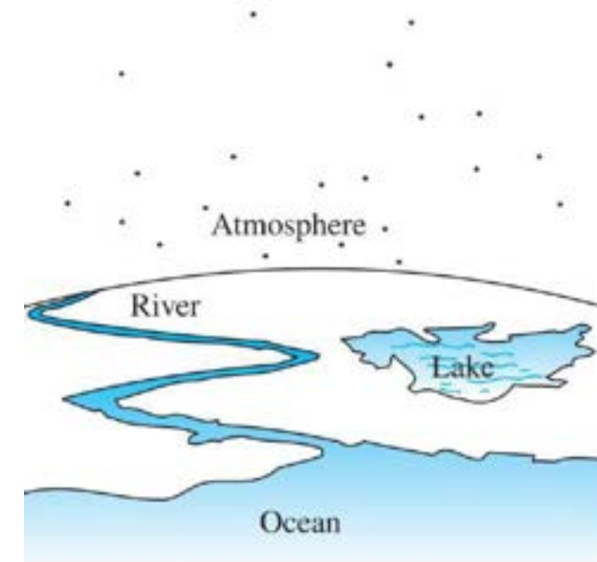
FIGURE Bodies with relatively large thermal masses can be modeled as thermal energy reservoirs.
